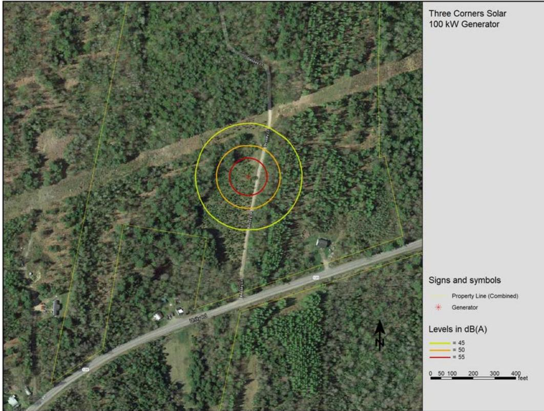
Figure 3 – Generator Sound Levels
