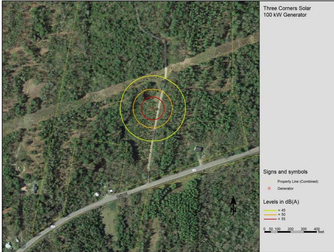
Figure 3 – Generator Sound Levels
